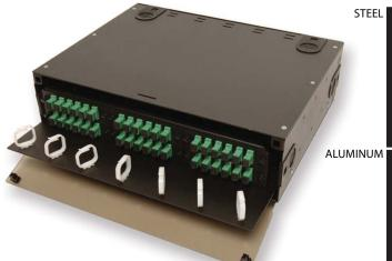
**Stock ID** 10-4538 (Black) 10-4541 (Off White) Description Rack Mount FDU 3RU in Height with 6 termination panel capacity and slide out master panel tray Dimensions 5.25" H x 17" W x 14.0" D Weight 24 lbs. .060" Powder Coated Steel
